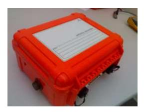
The eentec DR4050 ver. P is the latest version the rugged, *ultra low power*, *high-performance*, *versatile 24-bit seismic recorder line*. It is designed for the most demanding requirements in high performance seismic or strong motion research.
